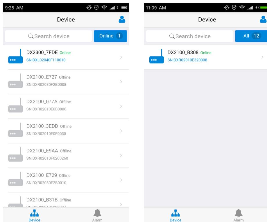
Device tab and alarm tab will be shown in the APP. In the device tab, the device information will be shown, include the value of registers of the remote device. And the value of the register can be changed in the APP as well. In the alarm tab, users can read the alarm messages.
