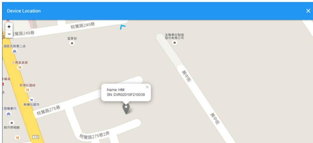
It will show the device name and SN of the device after clicking position icon in the map. When there is large number of device of user, it will switch to corresponding device when user clicks blue arrows at the edge of the map.
