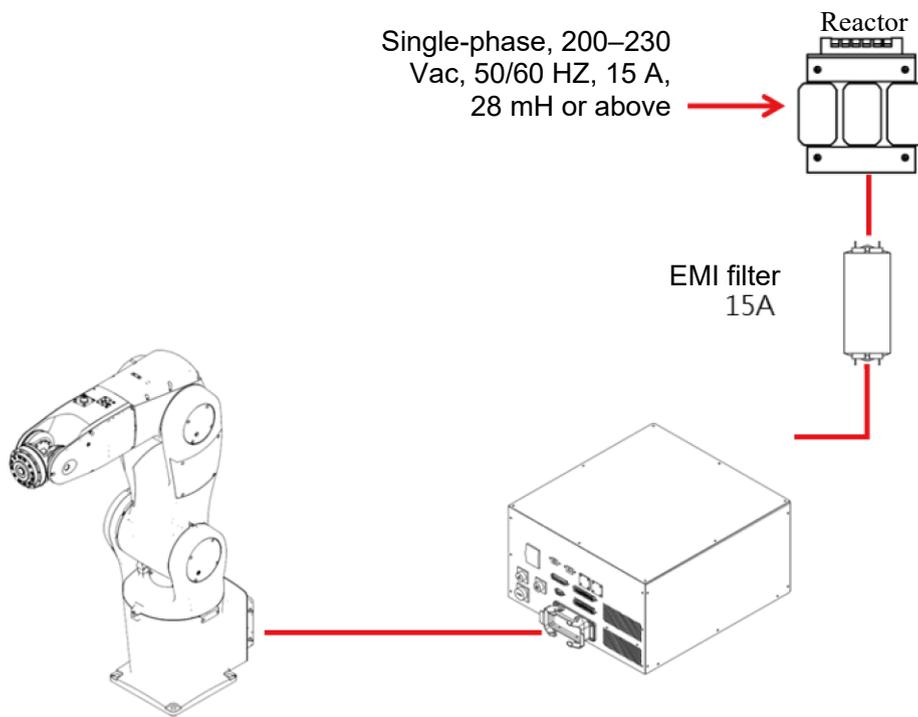
**Figure 5.4 Controller with EMI filter and electric reactor**
