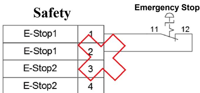
**Figure 5.17 Incorrect wiring for a single NC emergency stop**
