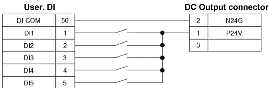
**Figure 5.33 PNP wiring when the input signal DI uses power from the DCV controller**
