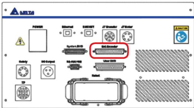
Figure 5.42 External encoder connector location
