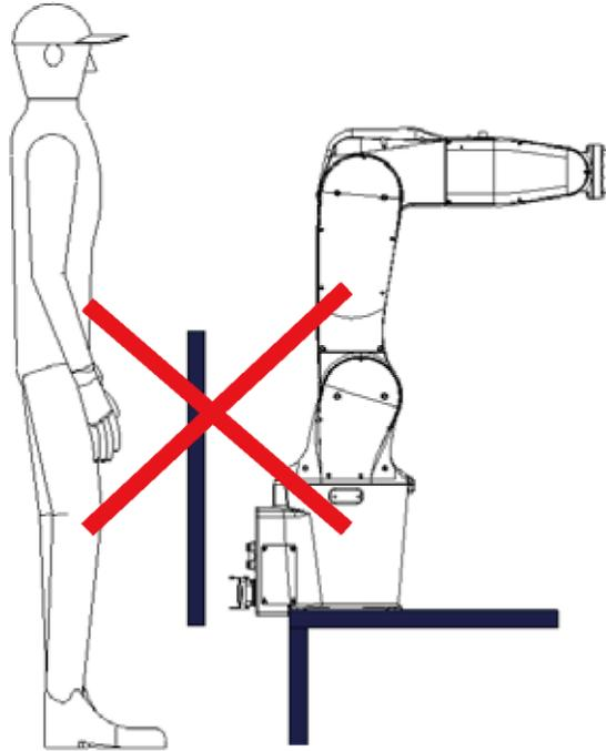
**Figure 4.6 Insufficient railing installation height**
