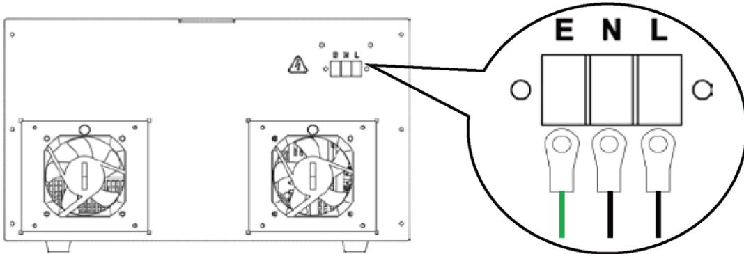
Figure 7.5 Quickstart wiring power wiring example
