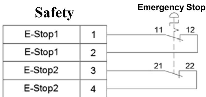
**Figure 5.16 Wiring example for a single Emergency Stop button**
