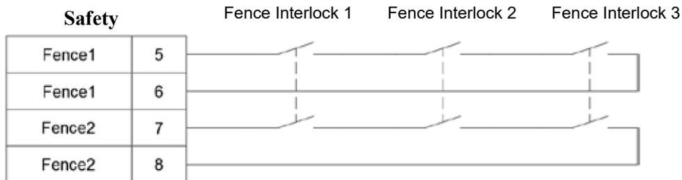
**Figure 5.20 Wiring diagram for multiple safety protection devices**
