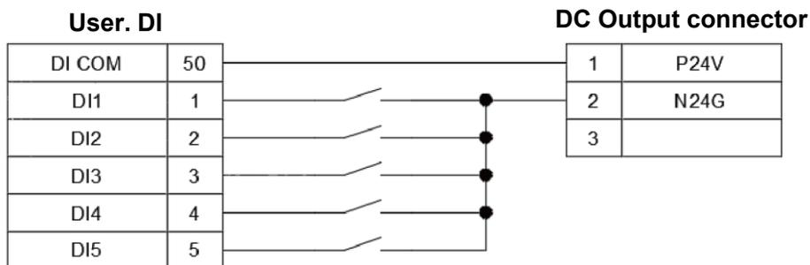
**Figure 5.32 NPN wiring when the input signal DI uses power from the DCV controller**
