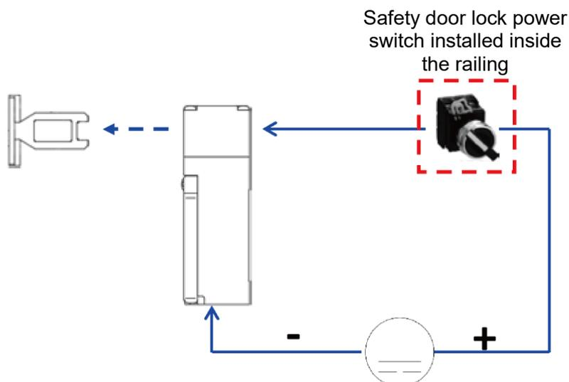
Figure 5.22 Electromagnetic safety switch wiring
