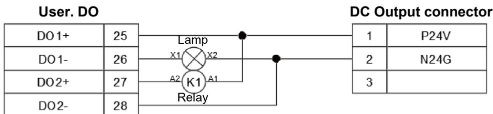
**Figure 5.38 User. DO DCV controller voltage mixed output wiring**
