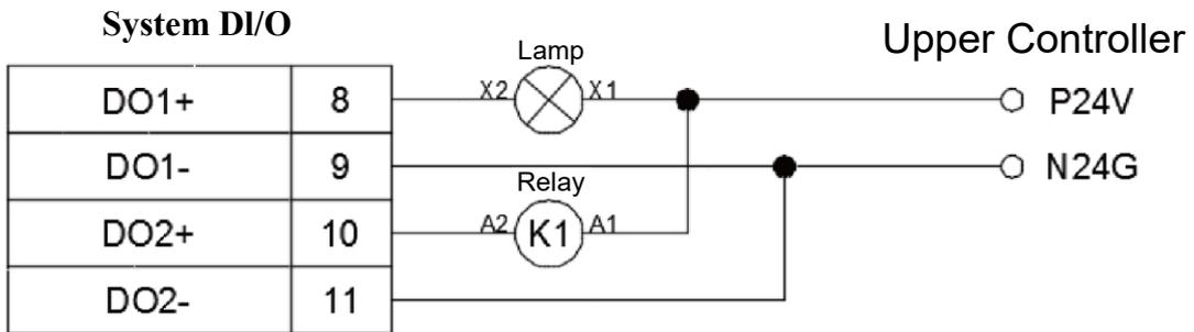
Figure 5.28 System DO upper controller voltage output NPN wiring
