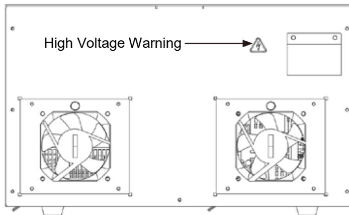
Figure 1.2 Sticker location on the back of the controller
