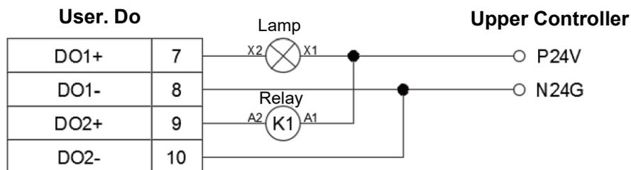
**Figure 5.39 User. DO upper controller voltage output NPN wiring**
