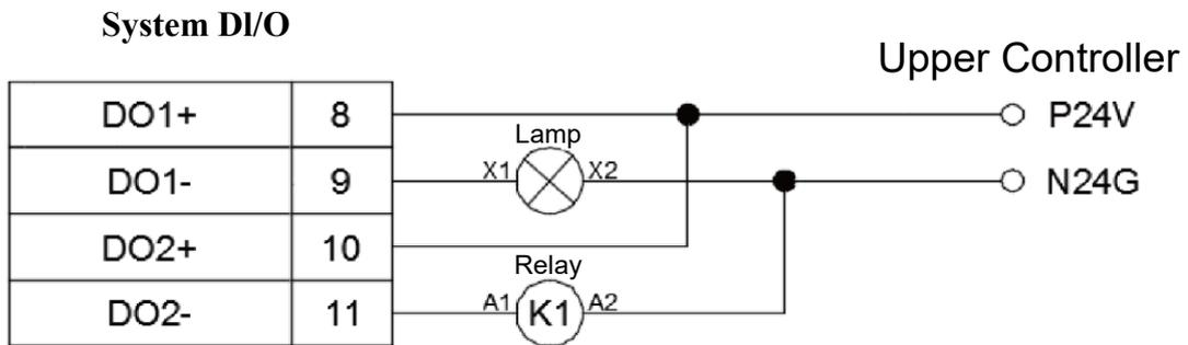
Figure 5.29 System DO upper controller voltage output PNP wiring
