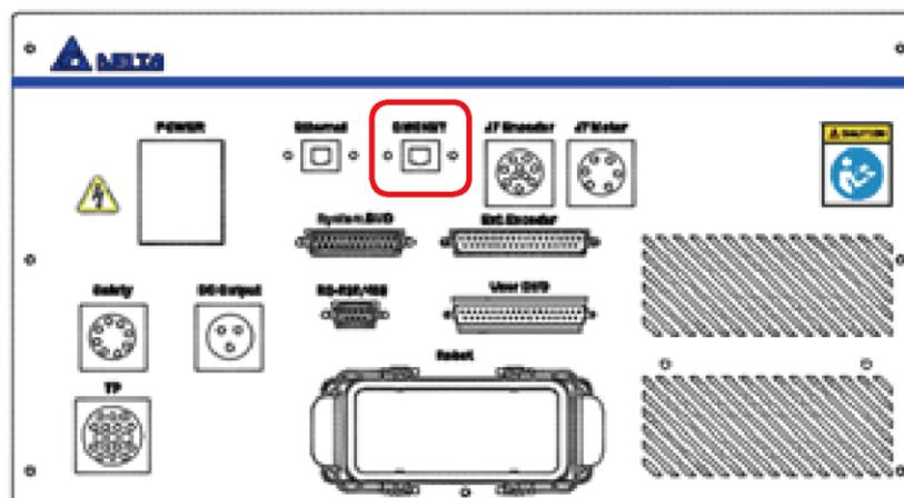
Figure 5.7 DMCNET connector location
