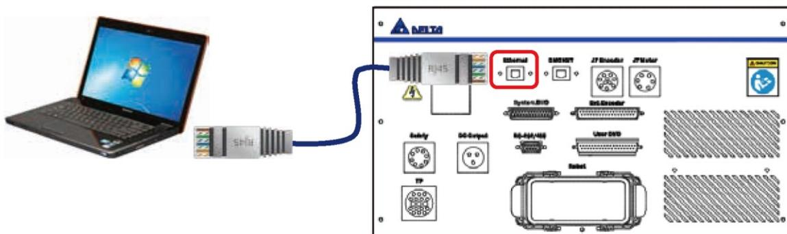
Figure 5.6 Ethernet connector location
