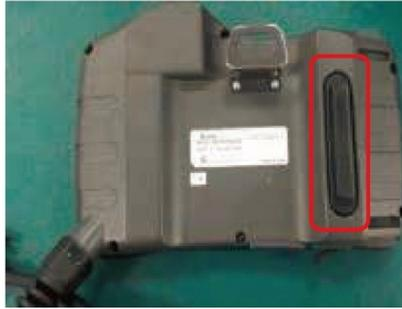
**Figure 5.13 Handheld teaching pendant Enable switch location**
