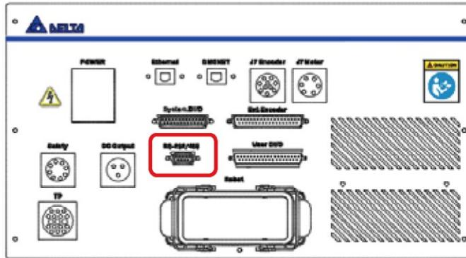
Figure 5.5 RS-232/485 connector location
