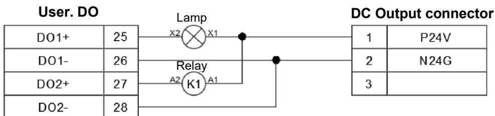
**Figure 5.36 User. DO controller voltage output NPN wiring**
