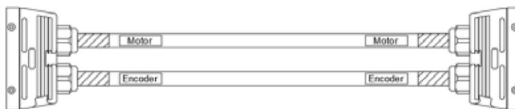
**Figure 9.8 Robot Cable**
