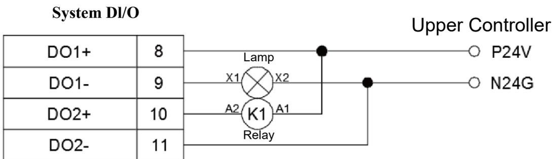
Figure 5.30 System DO upper controller voltage mixed output wiring
