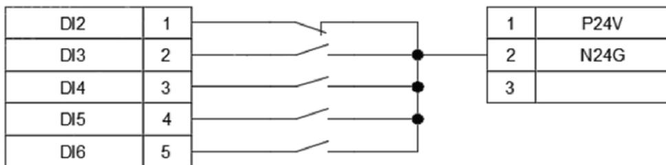
Figure 5.24 Input signal DI wiring
