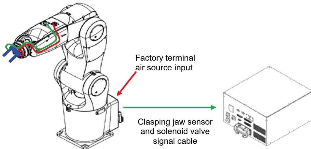
**Figure 6.6 Robot clasp jaw signal and DCV controller connection**
