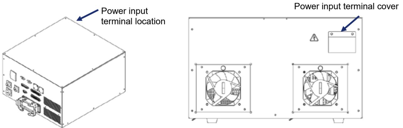
Figure 5.2 Power input terminal location
