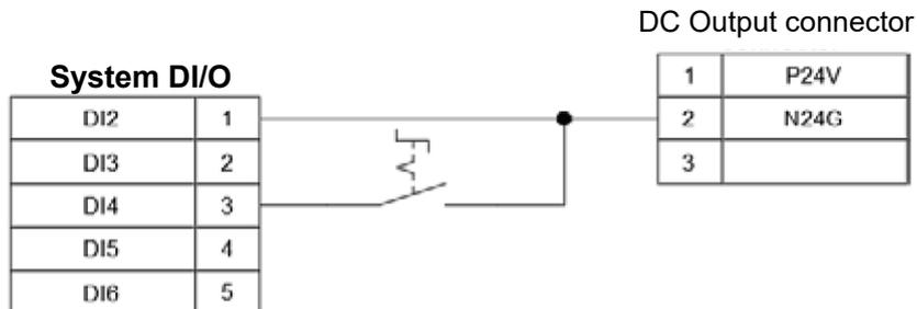
**Figure 7.4 Quickstart DI wiring example**
