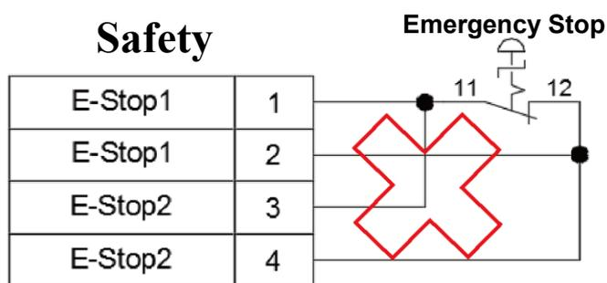
**Figure 5.18 Incorrect wiring for a single NC emergency stop with the safety signal connected**
