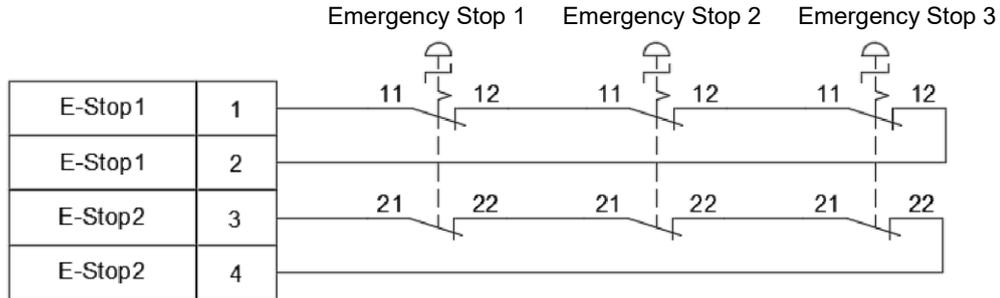
**Figure 5.19 Wiring example for multiple Emergency Stop buttons**
