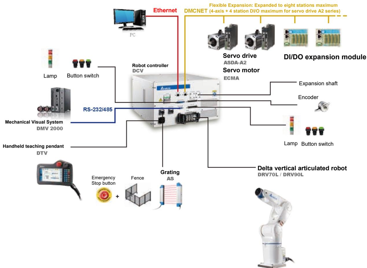
Figure 5.1 Controller peripheral system components
