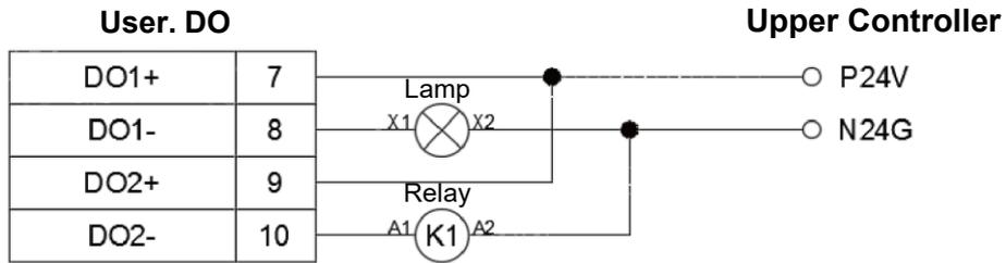
Figure 5.40 User. DO upper controller voltage output PNP wiring
