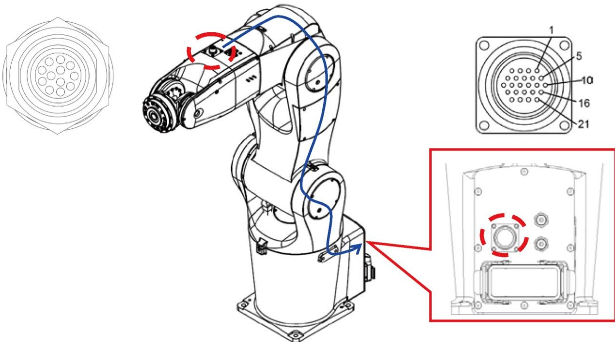
Figure 6.1 Internal wiring of the robot 12-Pos signal connector
