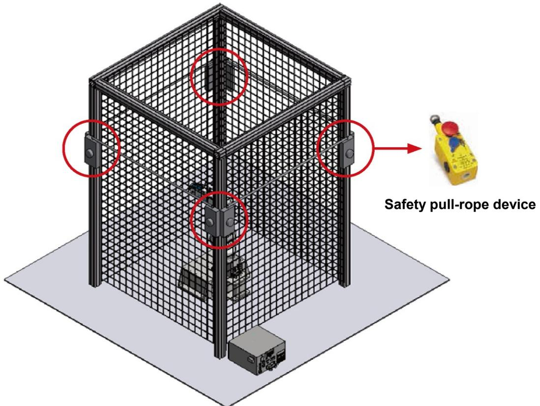
Figure 4.4 Safety pull-rope switch installation example
