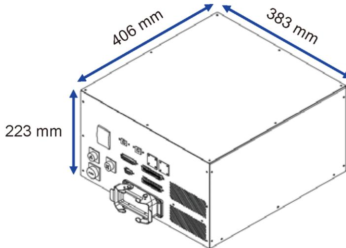
**Figure 2.1 Controller appearance and dimensions**
