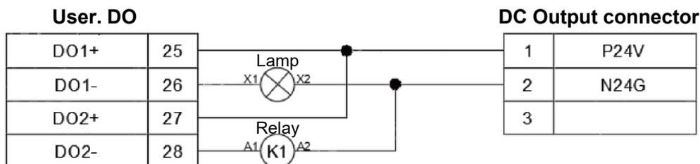
**Figure 5.37 PNP wiring when the input signal DI uses power from the Controller**
