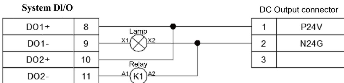
Figure 5.26 System DO controller voltage output NPN wiring
