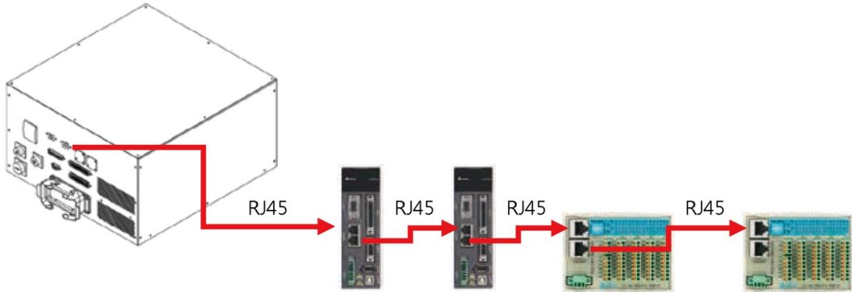
**Figure 5.8 Multiple DMCNET connections**
