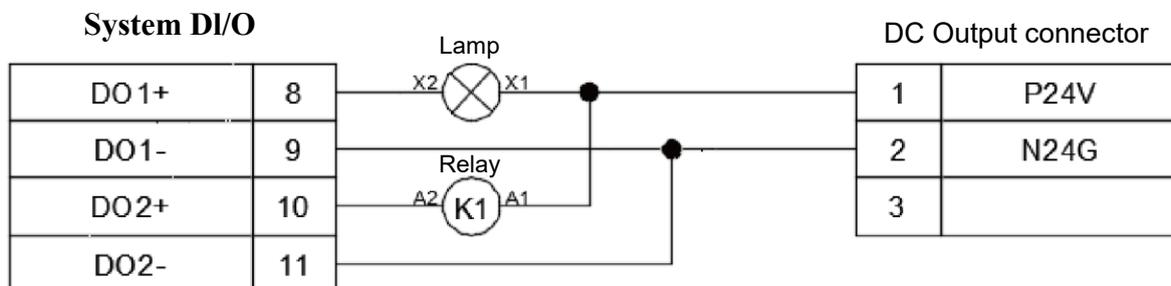
Figure 5.25 System DO DCV controller voltage output NPN wiring
