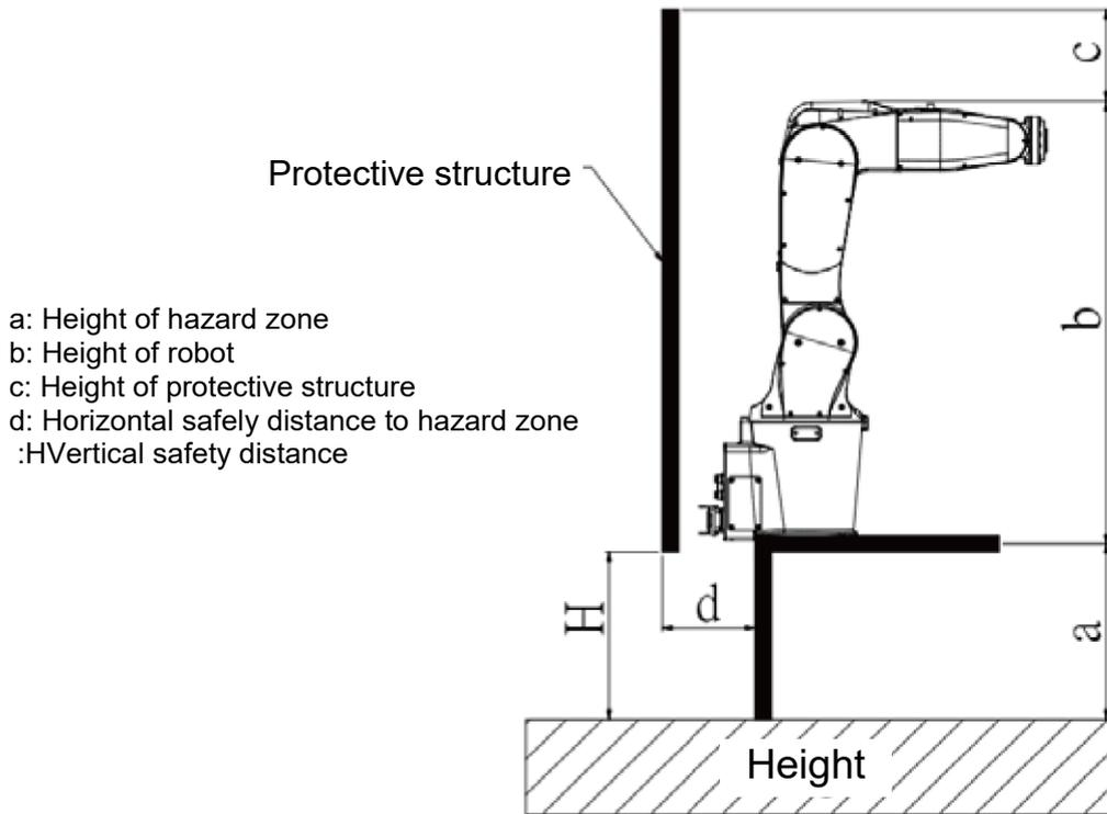
Figure 4.5 Installation height for railings around the robot
