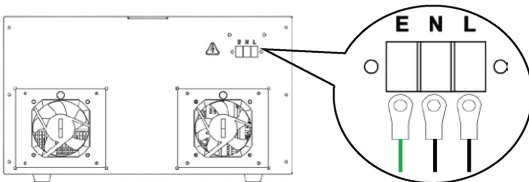
Figure 5.3 Power terminal wiring
