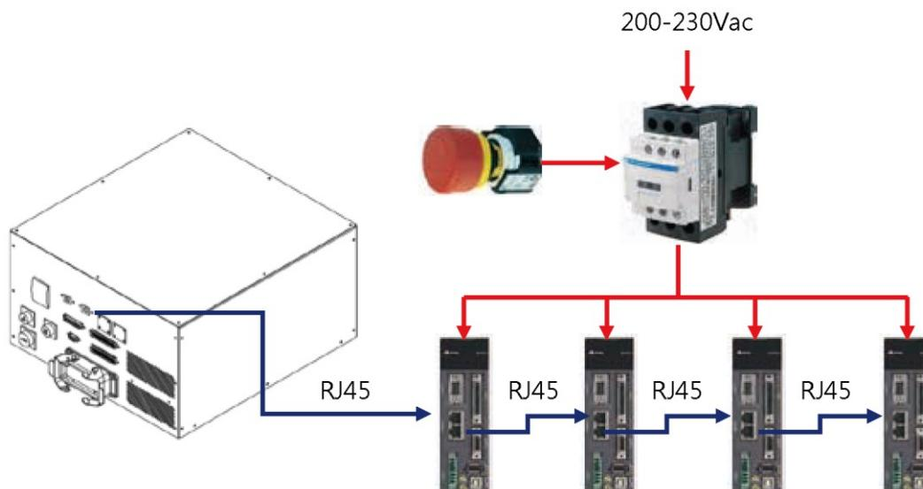
**Figure 5.9 Controller with external servo drive system architecture**
