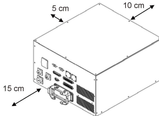
**Figure 3.3 Controller installation spacing**
