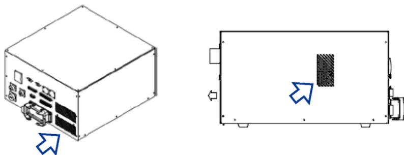
**Figure 8.1 Controller ventilation filter locations**
