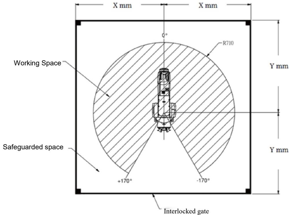
Figure 4.7 DRV70L safety grating installation distances
