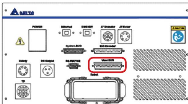
**Figure 5.31 User. DIO connector location**
