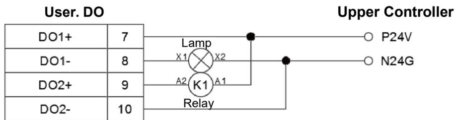
Figure 5.41 User. DO upper controller voltage mixed output wiring
