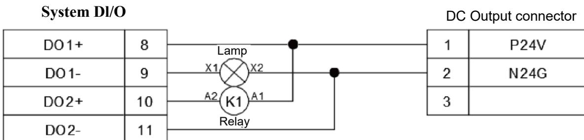
Figure 5.27 System DO DCV controller voltage mixed output wiring
