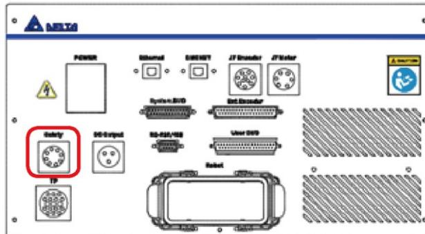
Figure 5.15 Safety connector location
