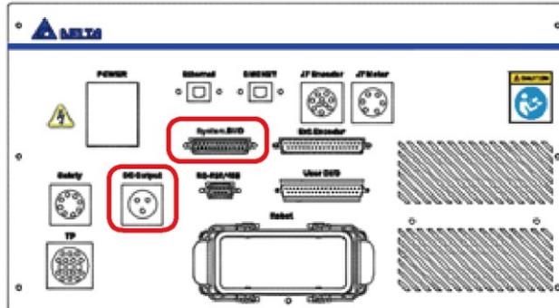
Figure 5.23 System .DIO and DC output connector locations
