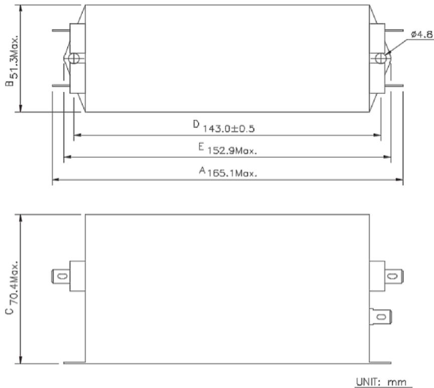
**Figure 9.1 Delta wave filter 16DPCG5-1 dimensions**
