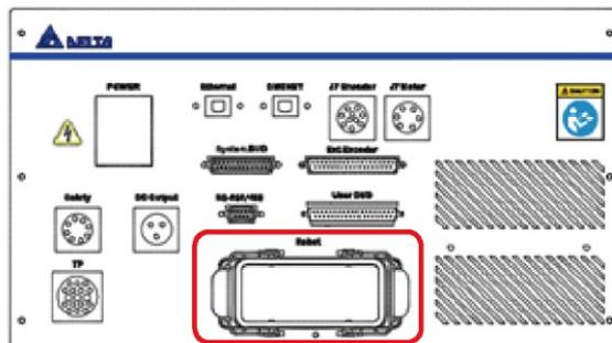
Figure 5.43 Robot cable connector location
