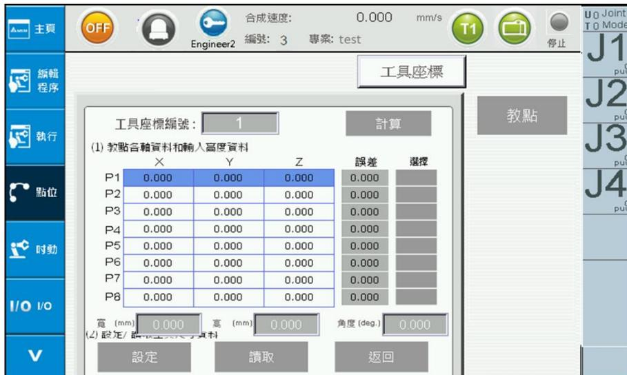
Figure 2-28 Point Information – Tool Size Calibration
