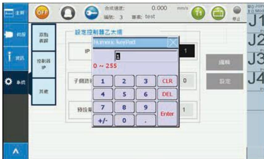
Figure 2-48 System Setting - Set Controller IP
