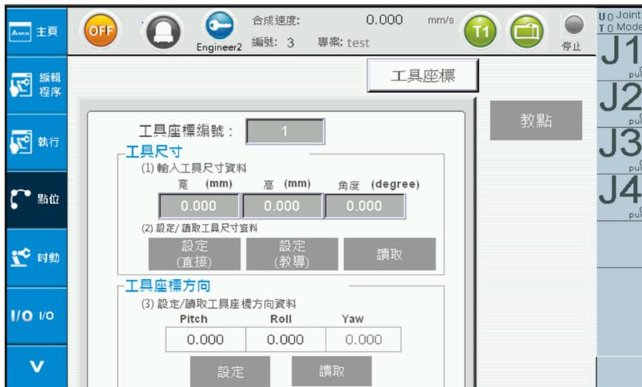
Figure 2-27 Point Information - Tool Coordinate Setting
