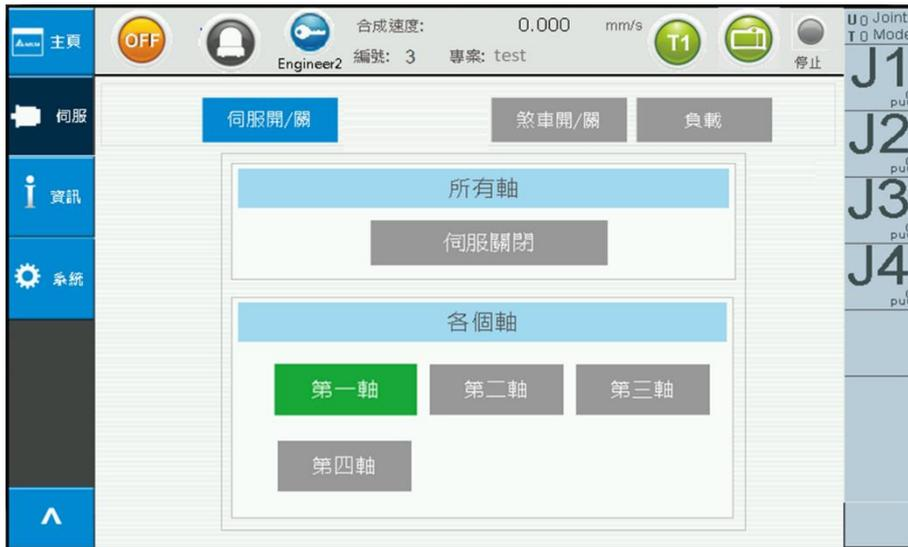
Figure 2-63 Servo Setting – First Axis Servo On
