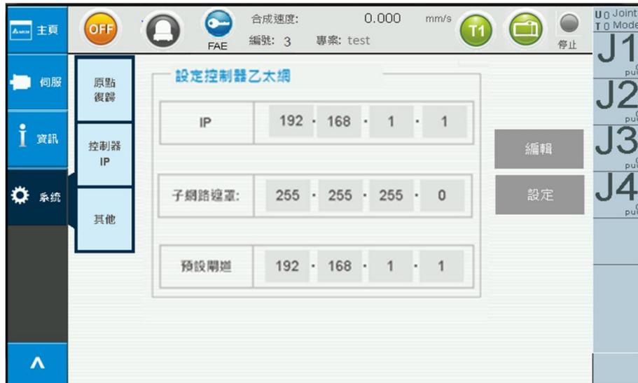
Figure 2-47 System Setting - Get Controller IP
