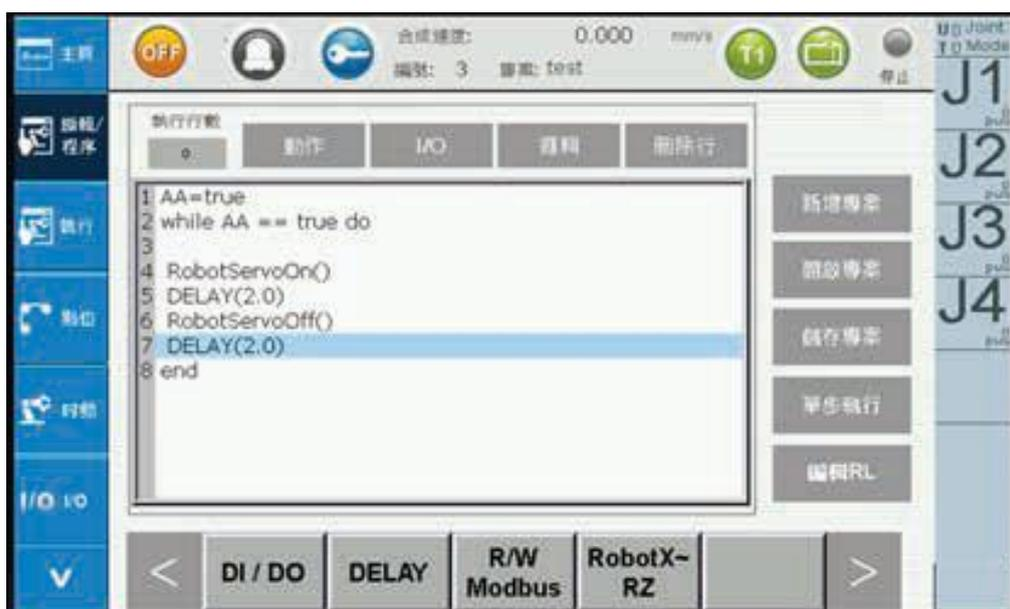
Figure 2-10 Robot Process Edit/RL - Program Opened
